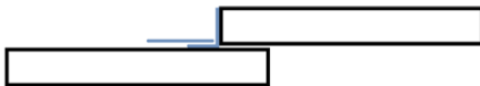
Figure 1: Aluminum Tape Installation Detail at Inner and Outer Layer Insulation Joints (tape shown in blue)
