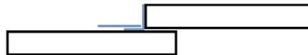
Figure 2: Aluminum Tape Installation Detail at Inner and Outer Layer Insulation Joints (tape shown in blue)
