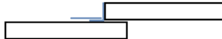
Figure 2: Aluminum Tape Installation Detail at Inner and Outer Layer Insulation Joints (tape shown in blue)
